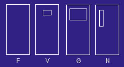
16GA (1.5mm),18GA(1.1mm),20GA(0.9mm) Cold-rolled or galvanized steel skins. Construction is 1-3/4" thick.
